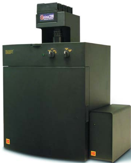
Gel Logic 2200 System with 2.2 megapixel cooled CCD camera and multi-purpose imaging cabinet
